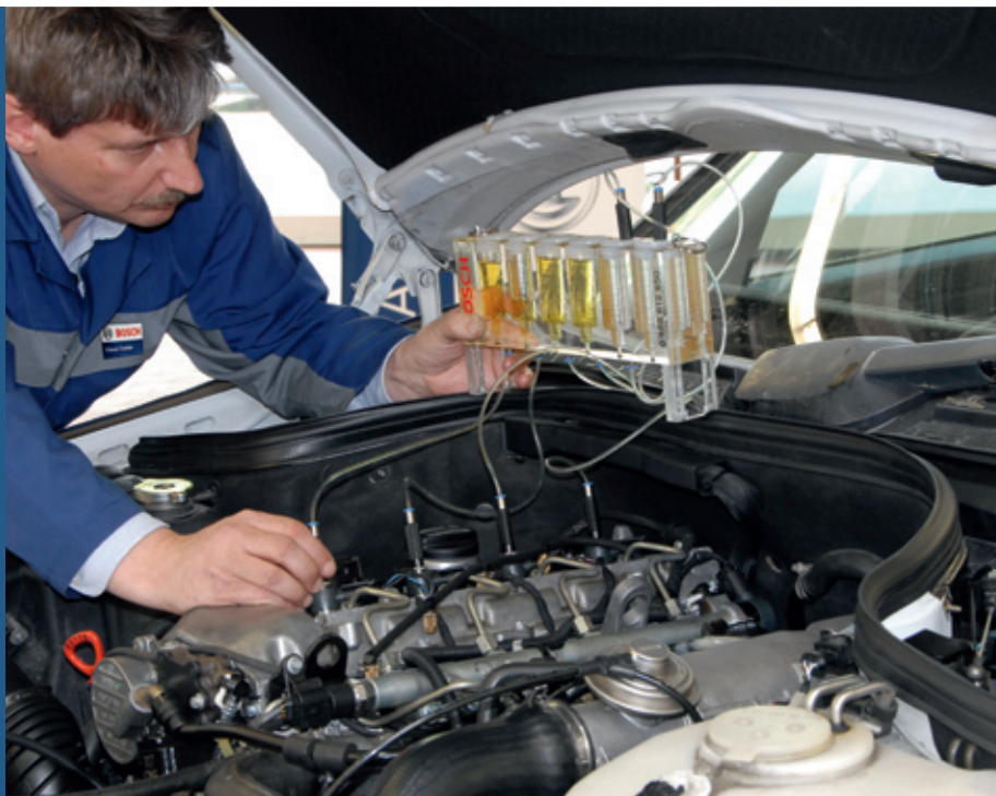
Measuring return quantities exposes defective Common Rail injectors. Photo: Linzing
