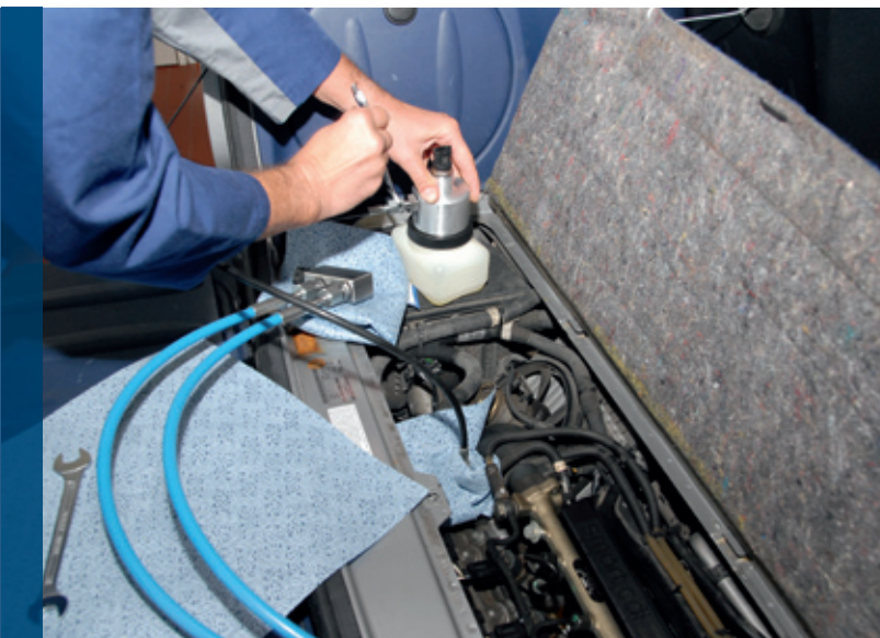
The pressure sensor module allows the specialist to test Common Rail pressure during start-ups under real conditions.
